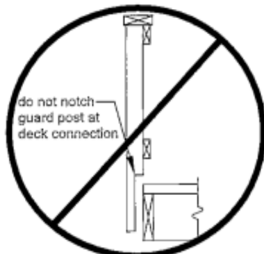
FIGURE 28: NOTCHING AT GUARD POSTS
